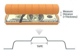
Signal of SBM tape detecting sensor
